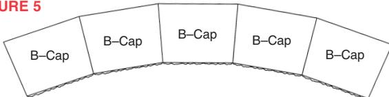
On all but the tightest curves, some gapping at the back of the caps will be needed to match wall alignment. Do not adjust caps by gapping at the front; the front joints between caps should be kept tight. Generally, gaps of up to 1/2-inch at the back of the cap units are considered acceptable. To completely eliminate gapping on most curves, saw-cutting the sides of cap units may be necessary. (See Saw-Cutting Caps Units section).
