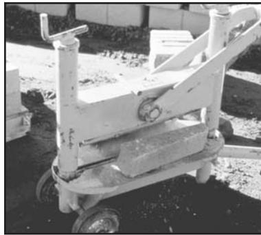
To split a cap, score the top and bottom of the cap with a chisel at the location and angle of the needed split. At the scored line, split the cap unit with a hammer and chisel. A minimum split thickness of two-inches is needed for an accurate split. Alternately, a mechanical splitter can be used.
